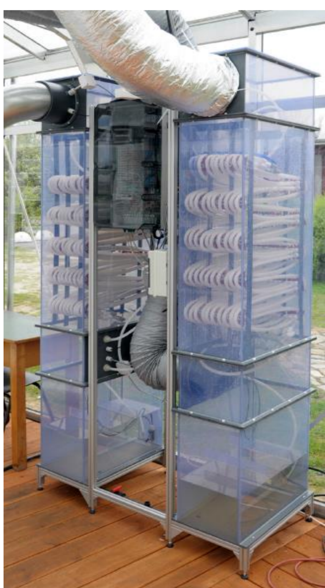
Figure 3: absorption concepts tested in Wangen: absorption box of Watergy, absorption box with packing materials, open system without ventilation
